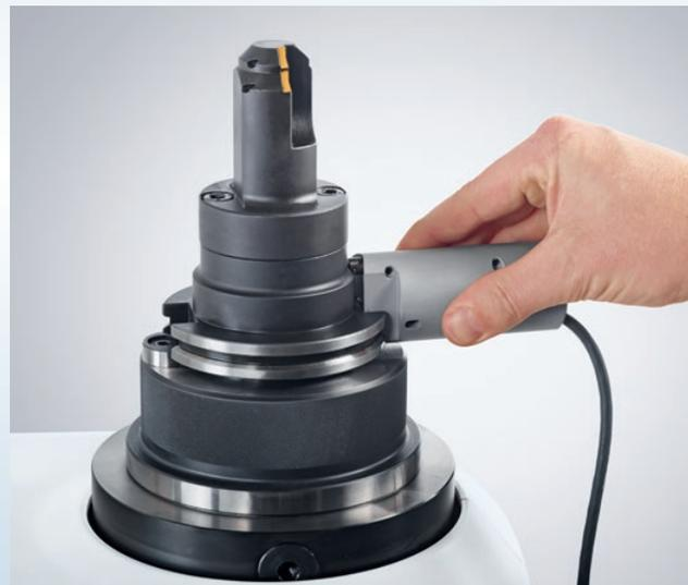
Manual positioning of the read/write head
